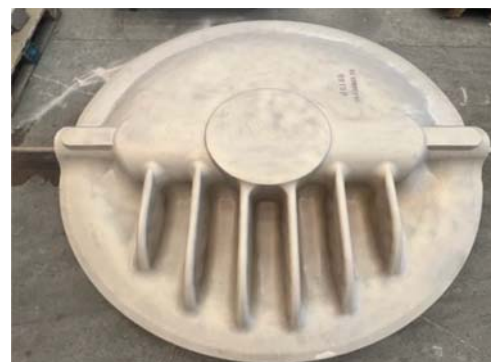
Figure 1. DN 2800 Disc - 5720 kg 'as cast' weight.
