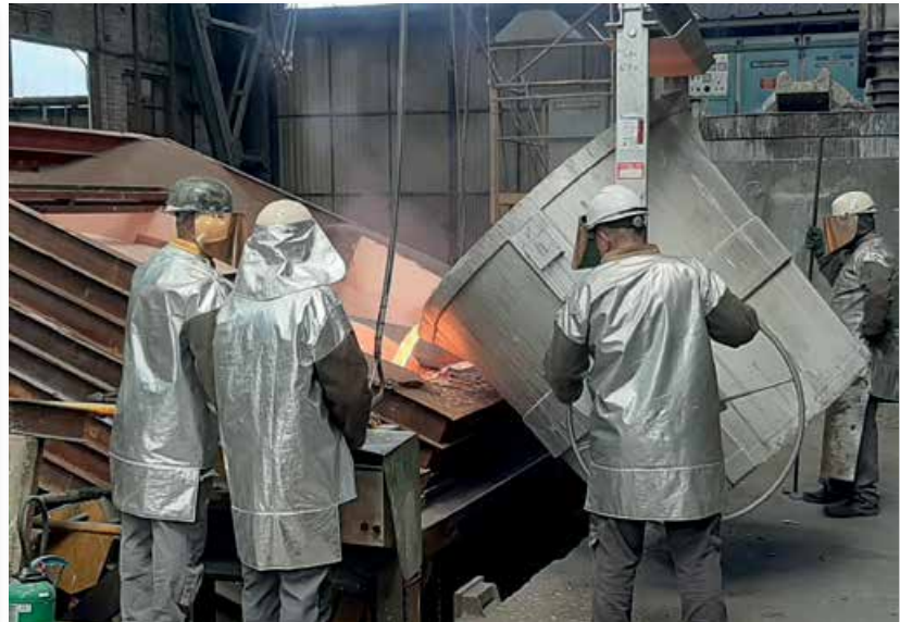
Pouring 6To of alloy in 3D sand printed mould @ 1 250°C (Inoxyda).
