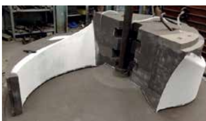
Segment 1 of pump hydraulic (Inoxyda).
