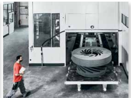
Large size 3D sand printed cores (VoxelJet VX4000).
